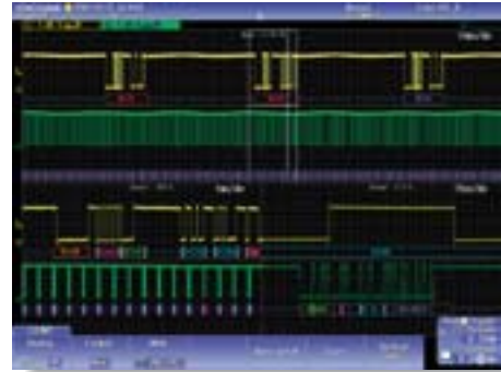
Simultaneous analyses of CAN and LIN
