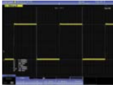
Simultaneous level and time difference measurement with the \Delta T \& \Delta V cursor
